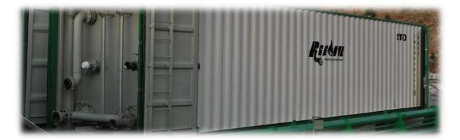
Designed to work in conjunction with Reform Energy Services UBD/MPD package, our closed top cascading 400 bbl storage tanks will enhance the separation and subsequent removal of any poisonous gas from the system. Additionally, they will act as a retention vessel generating a cleaner and solid free drilling fluid.
