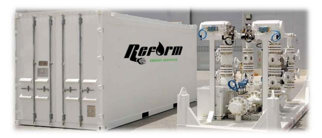
Reform Energy Service's MPD manifold has been designed to automatically maintain the annulus surface back pressure during drilling operations to maintain the downhole drilling window. It uses two drilling chokes which are controlled by a PLC control system to maintain the selected set point pressure using an HMI interface panel for operator input of required settings and for displaying control system output parameters. If required the manifold can also be used in a manual mode.
